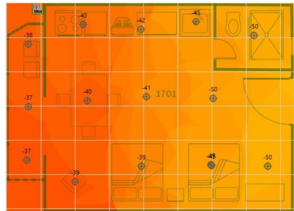
Fig. 4. Wi-Fi intensity test in room 1701. Source: Own elaboration of the author.
