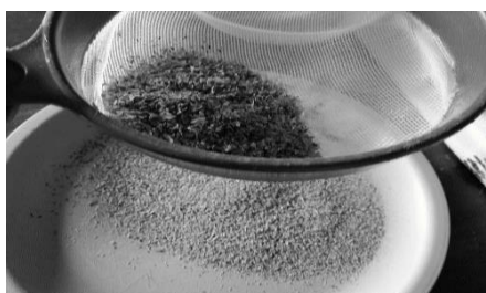
Fig. 8. Sifting of the powder resulting from grinding.
